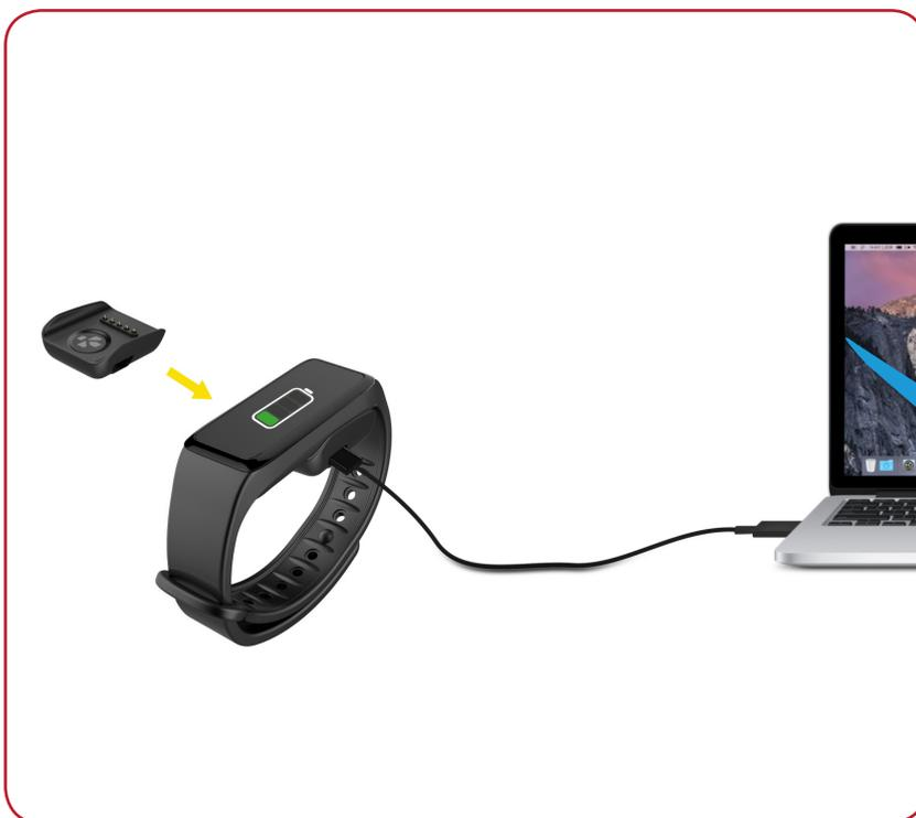
Before the first set-up, we recommend you to charge your ZeFit<sup>3HR</sup> for about 1h30. Make sure to well align the charging clip posts with the contacts on the back of ZeFit<sup>3HR</sup>. Plug the USB cable to a power source. A battery indicator will be displayed on the screen.
