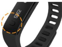
Click and hold down the main button of your ZeFit to switch on the screen and enable the connection between the two devices
