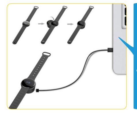
Before the first set-up, we recommend you to charge your ZeCircle for about 1h30. Make sure to well align the charging clip posts with the contacts on the back of ZeCircle. Plug the USB cable to a power source. A battery indicator will be displayed on the screen.
