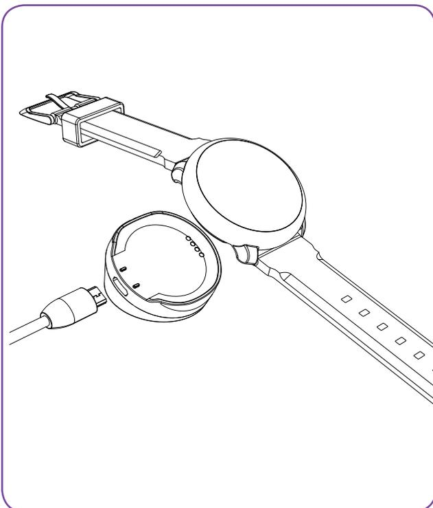
Before the first set-up, we recommend you to charge your ZeRound for about 2 hours. Make sure the pins on the cradle fit correctly onto the charging terminals on the back of the device. Plug the USB cable to a power source. A battery indicator will be displayed on the screen.
